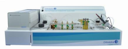
Figure 6. OI Analytical FS3700 Automated Chemistry Analyzer for ASTM D7511-09e2
